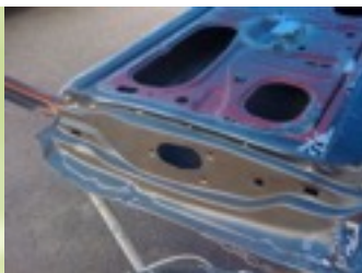
Car door with paint removed back to bare metal. No pitting.
