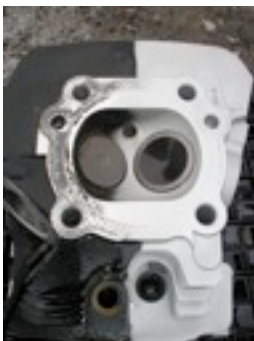
Motorbike engine with half of carbon build up removed.
